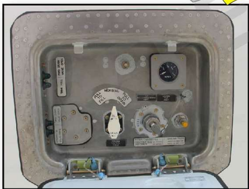
POTABLE WATER SERVICE PANEL
