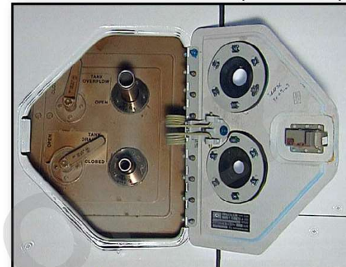
OVERFLOW/DRAIN PANEL (A320 ONLY)
