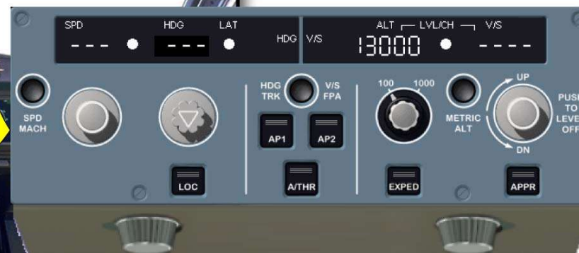
Flight Control Unit (FCU) (13VU)
