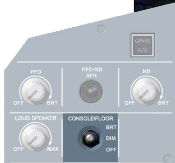
EFIS CONTROL PANEL (301VU)
