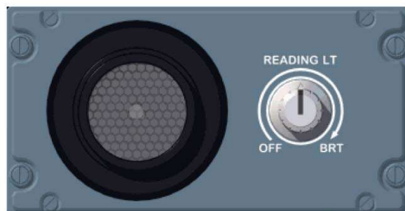
READING LIGHT PANEL (54VU)
